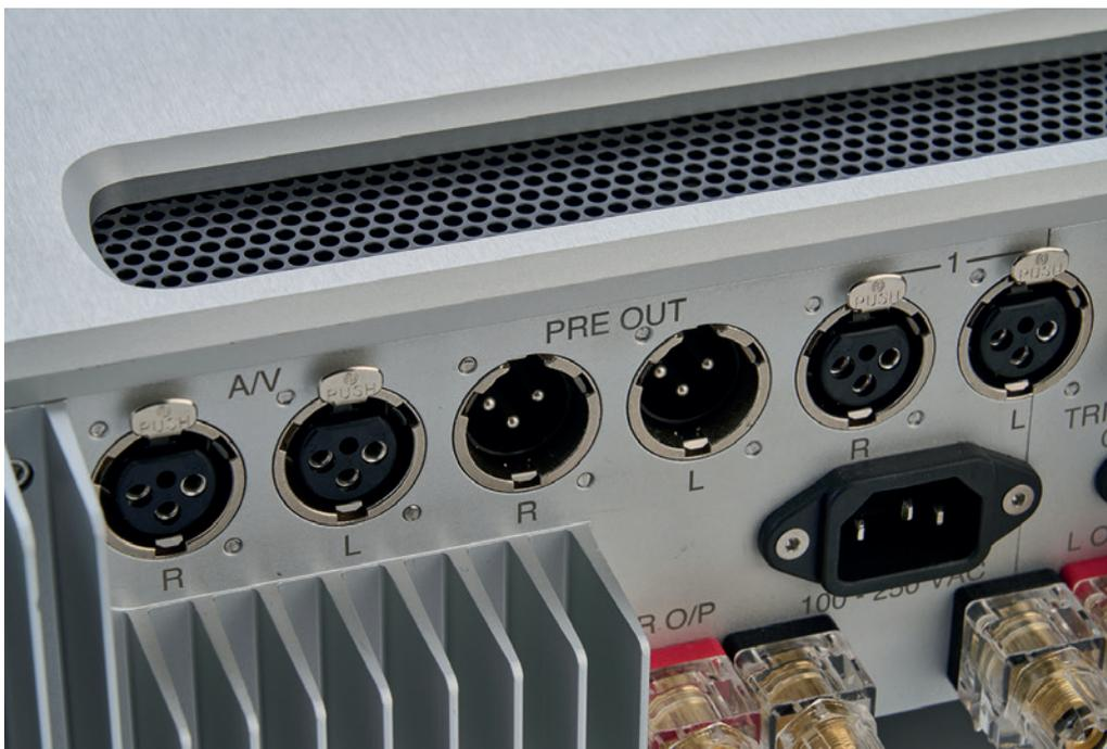
*Shown here is the balanced connector section: AV input for integration into a surround system, preamplifier output, but only one pair of balanced inputs*
