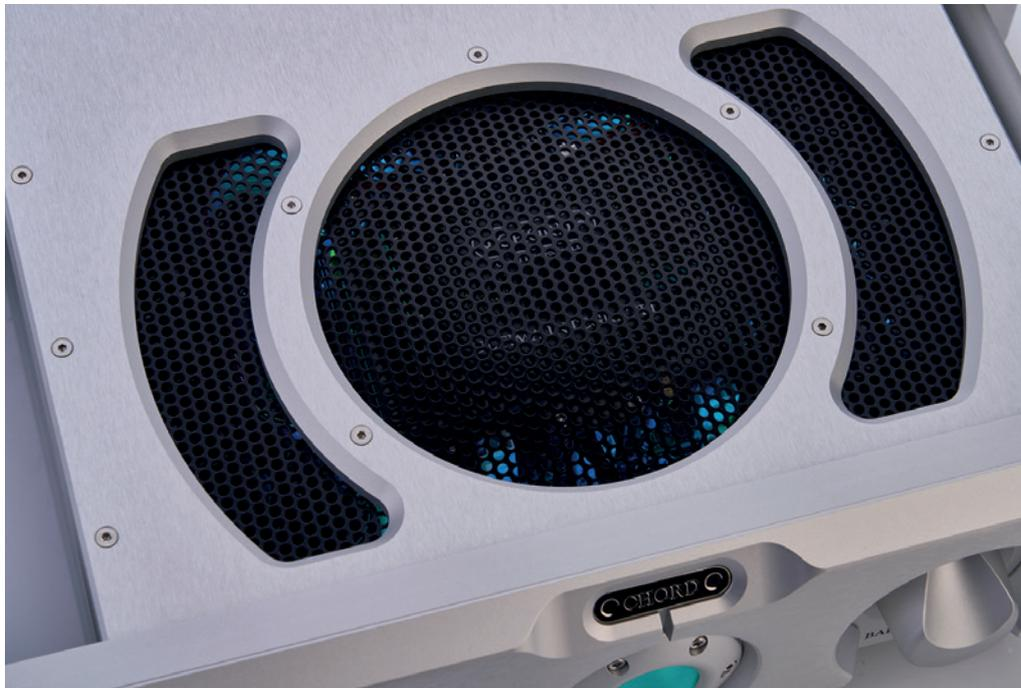
*The well-designed openings at the top of the Ultima Integrated are used for cooling, but also allow the light from the LEDs to shine through in a green-blue colour*
